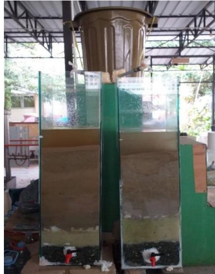
**Gambar 1.** Rangkaian Unit Alat *Biosand Filter*
